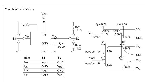
Notes: 1. Waveform - A is for an output with internal conditions such that the output is high except when disabled by the output control.
